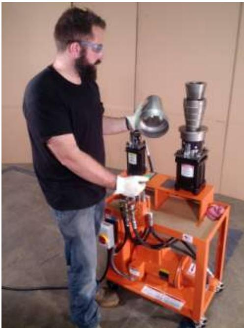
The new 1674V Expander has two expanding cylinders mounted vertically. According to company president, Ken Murray, “The vertical orientation has two sets of benefits. One, many fabricators like working this way, in essence using gravity to hold the part against the expander head. The second benefit is that you can use larger segment sets, and get wider expansions. We have made this as a custom machine for the last few years, and we have customers expanding up to 12 inches.”
